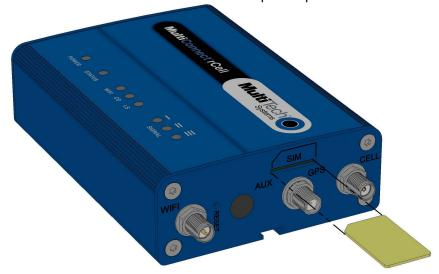
3. To remove the SIM, push the edge of the card in. When released, the card pops out of the device.
