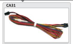
Main port extended installation cable with an 8pin double row, UCOM connector and open ends. Open wires (6pin): 3 x IOs, IGN, V+, GND
