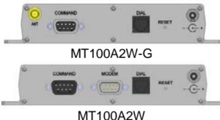
1. Connect a suitable antenna to the ANT connector on the MT100A2W-G model.
